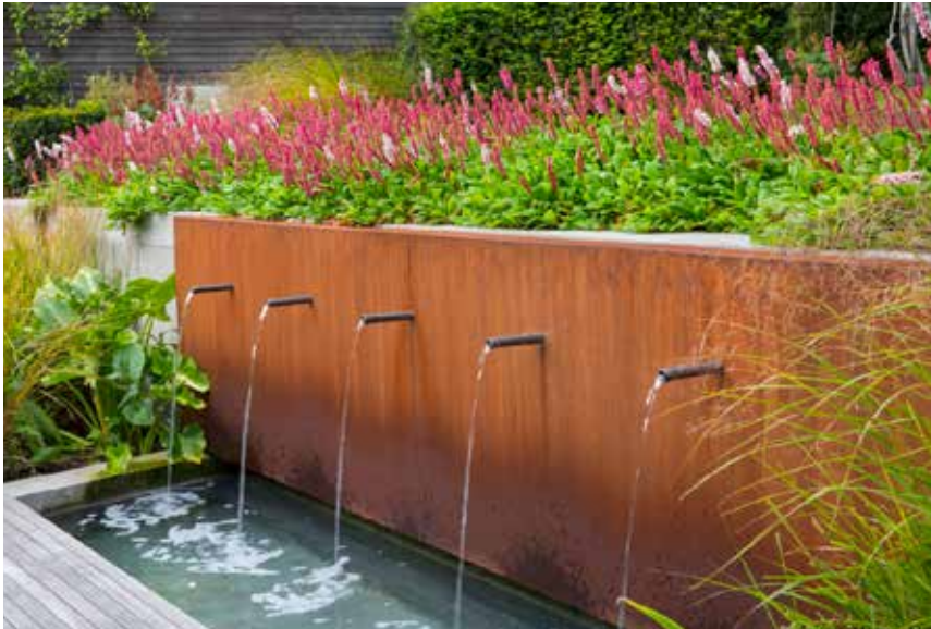
The planting bed is lined with a geotextile membrane and then filled with a layer of drainage material topped with lightweight soil. The utilitarian copper spouts (actually gas piping) will turn verdigris in time and stand out against the rusted steel.
